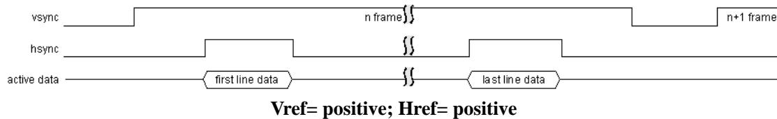
In the valid area of Vsync and Hsync, making the data sample through pclk and buffering the picture data to dram
