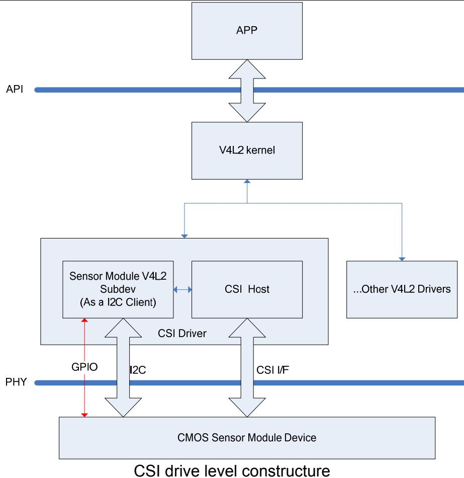
CSI drive is designed based on Linux V4L2 framework and can meet the standard V4L2 API calling mode. Because the data buffering of CSI hardware collection requires physical continuous internal memory, the video-dma-contig internal memory way is applied for the management.
