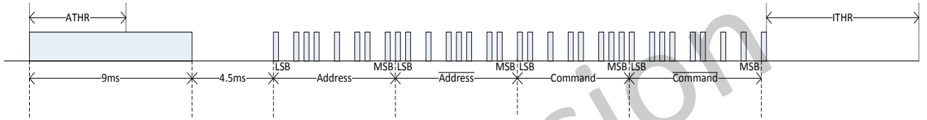
Figure 9-111 NEC Protocol
